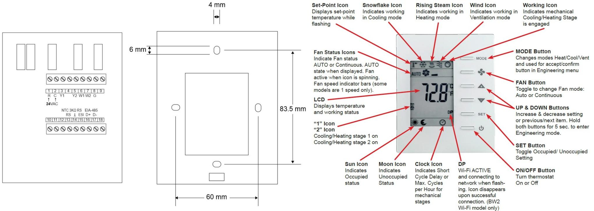
The BASstat has a built-in space temperature sensor with provision for remote wired 3kΩ NTC thermistor sensor or temperature value can be sent by another device over the BACnet network.
